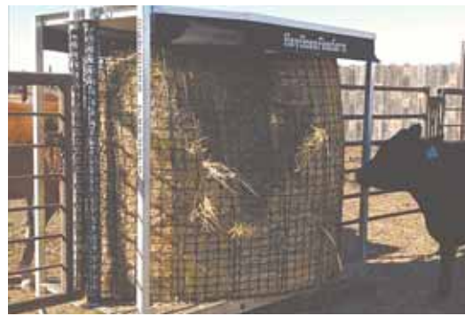
HayBoss Feeder is fitted with vertically suspended, retractable polypropylene nets. Mounted on self-tensioned, spring-loaded rollers, the nets form a cradle to snugly hold the feed and prevent waste. Models are available for both round and small square bales.
