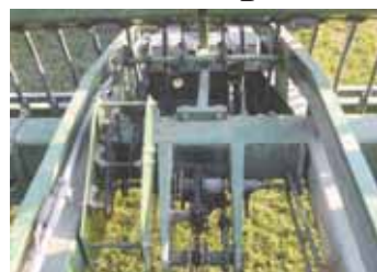
He installed the grass seeder off a Deere 750 grain drill on front of the planter and also built a transmission to run the seeder.
