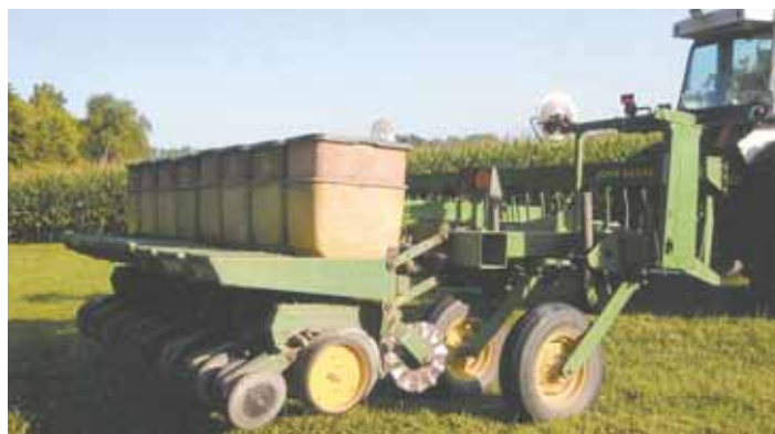
Richard Lindemer built this bean planter out of a Deere 7000 wide-row corn planter. He uses it to plant beans in the spring and cover crops in the fall.
