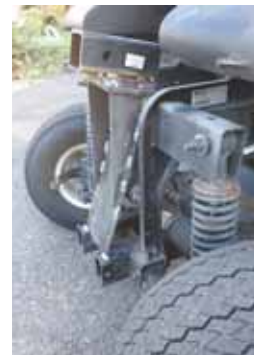
Bracket keeps receiver hitch high off the ground, putting the load's weight on the axles.
