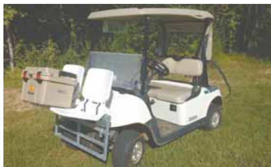
Front-mount receiver hitch allows attachments to be added to golf carts, such as the 2 safari seats shown here.
