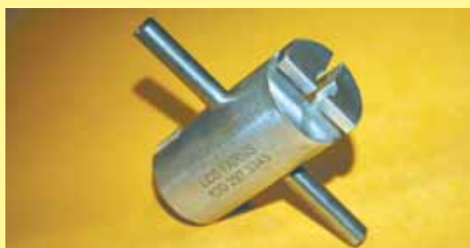
The tool makes a tightly wound splice that conducts electricity as well as unbroken wire. Splicer is made from aircraft aluminum to keep it light and free from rust.
