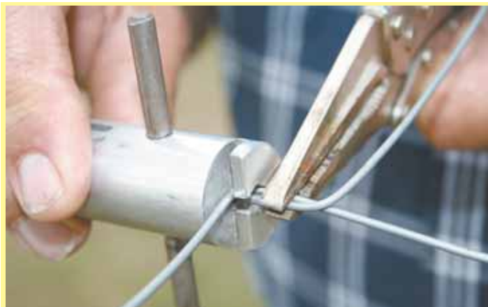
Using the Wire Splicer requires an overlap of about 6 in. of wire, and a needle-nosed vicegrip to hold the wire tight during splicing.
