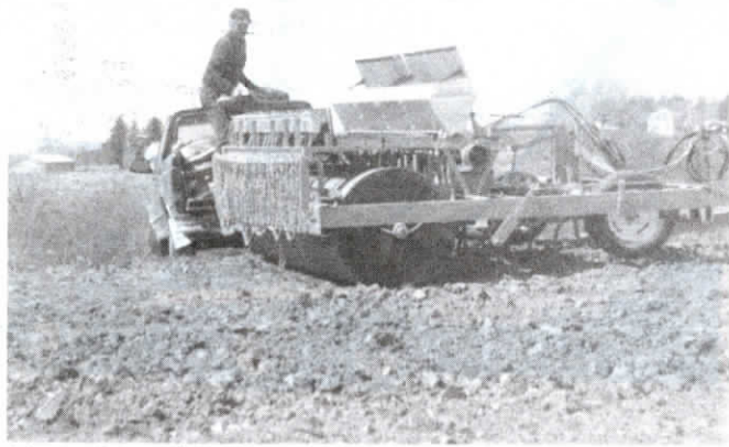
Johnston plants grains and beans out of front drill boxes and alfalfa or grass seed out the back. Seed from both boxes drops out of tubes that end about 14 in. above ground.
