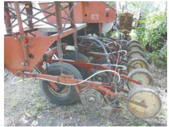
He reinforced the planter's rockshaft and added a second set of wheels to support the added weight of liquid fertilizer.
