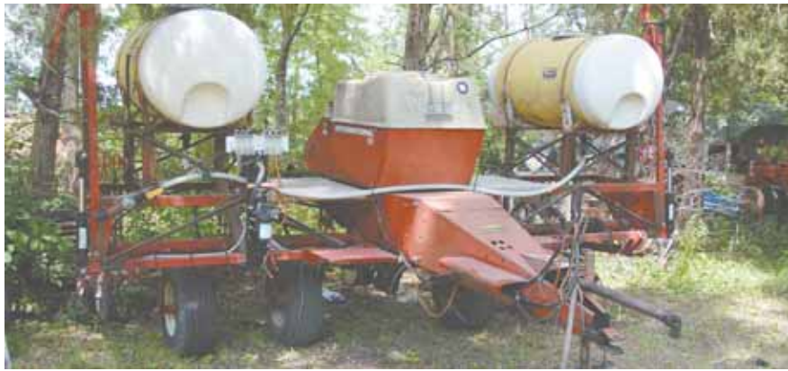
Mike Bauer rebuilt this 40-year-old, 6-row 400 IH Cyclo corn planter, replacing the dry fertilizer tanks with 2 fiberglass tanks that hold 125 gal. each.
