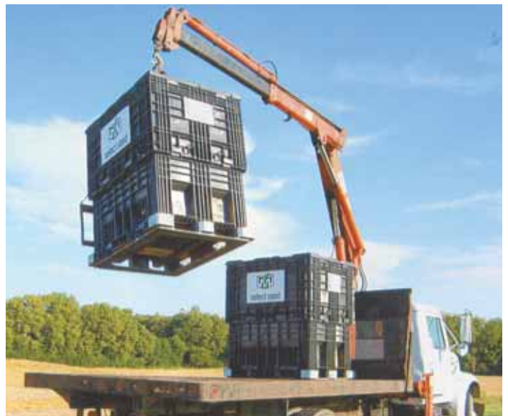
Greg Weaver uses his IH mid-mount “boom truck” to load Pro Boxes of soybean seed into his no-till drill. He also uses the truck to deliver seed to customers and to load and move machinery and lumber.
