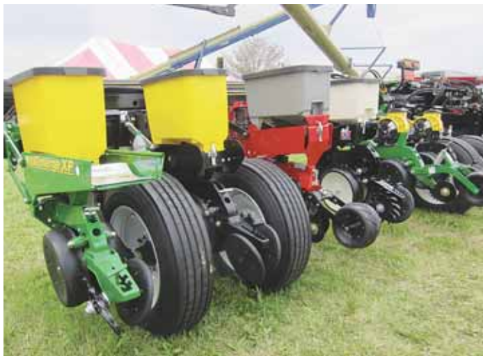
A Harvest International toolbar was fitted with colored planter row units at a recent show, each representing a different manufacturer. Precision Agri Services says farmers can save money with custom-built planters designed for precision agriculture.
