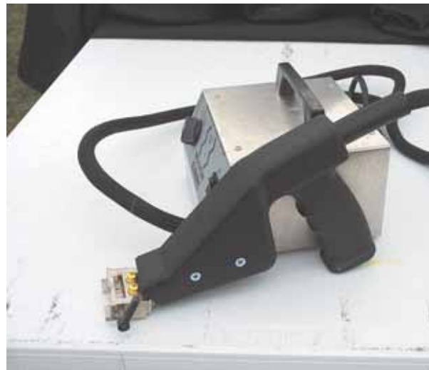
Nextire grooving gun heats a horseshoe-shaped razor blade that creates grooves in tire up to 1-in. wide and 1-in. deep.
