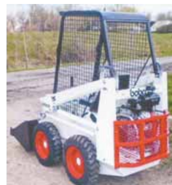
Leonard Wulf replaced the 13 hp Kohler engine on his 1973 Bobcat 371 skid loader with a 20 hp Honda V-Twin engine.
