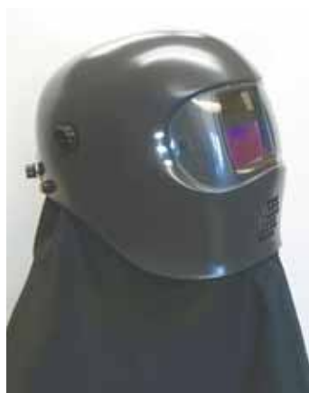
WindMaker welding helmet pulls air from the rear through a filter and directs it forward for breathing. A second fan near the chin pushes out stale air.
