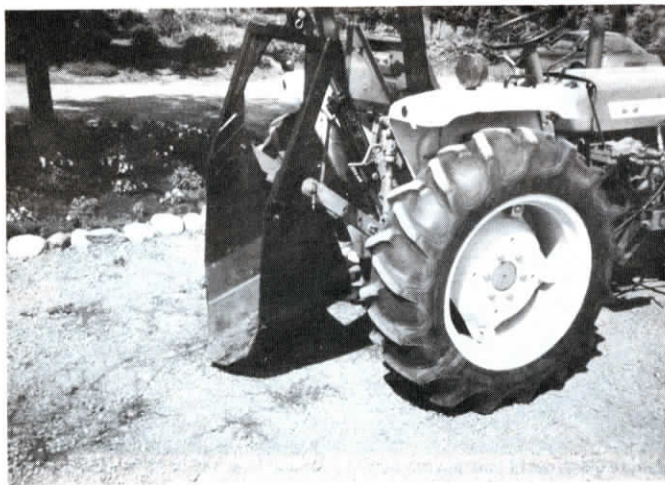
Digger's U-shaped blade is open on both ends. When 3-pt. mounted it can dig as deep as 24 in.
