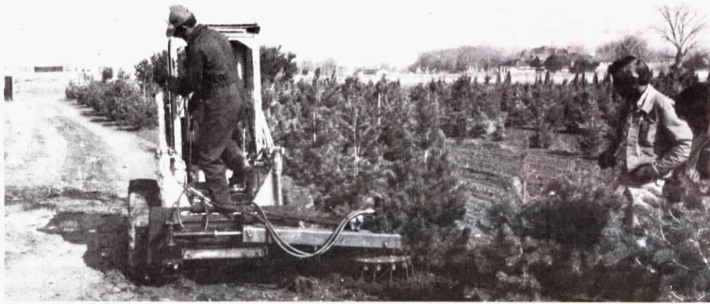
Weed Badger adapts to all skid steer loaders, and to tractors as a rear (3 pt. hitch) or side mounted (either right or left) unit.
