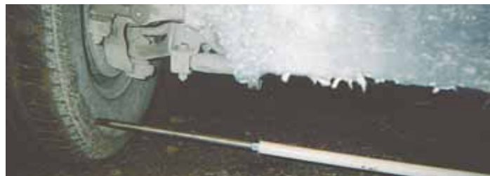
A 27-in. long threaded rod fits inside a 44-in. length of threaded pvc pipe. A nut and washer serves as a spacer and allows the threaded rod to be adjusted in and out.
