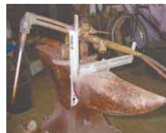
"With my anvil-mounted 'torch holder', I always have access to heat while forging small parts," says Robert Stone.
