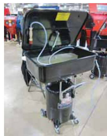
BadBoy parts washer uses your existing air compressor, saving the cost of replacing electric motors that plug up with grease.
