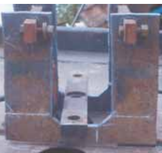
U-shaped "blade bar puller" makes it easier to remove the blade bar from the gearbox on a bush hog mower.
