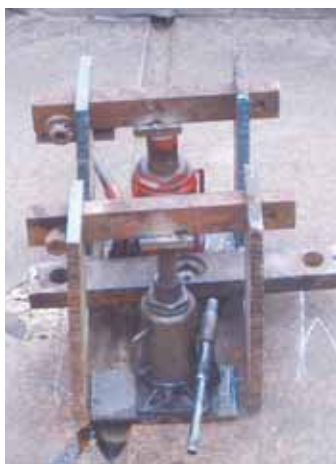
U-shaped "blade bar puller" makes it easier to remove the blade bar from the gearbox on a bush hog mower.
