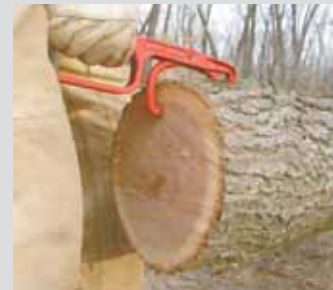
LogJaw log carrier has a steel hand that grips the wood with 3 sharp points and holds it tight.
