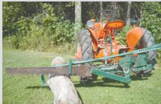
Wilmer Hanson is still using his "best buy" 1942 Ottawa pto-driven drag saw.
