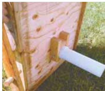
Juice is spun out of drum through pipe. It drains into a plastic pail, which is fitted with a screened lid to catch any larger bits of apple expelled with the cider.
