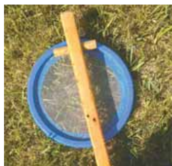
Juice is spun out of drum through pipe. It drains into a plastic pail, which is fitted with a screened lid to catch any larger bits of apple expelled with the cider.
