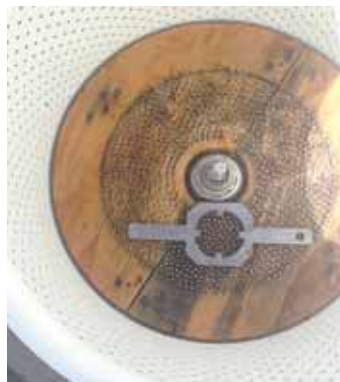
Philemon Riehl converted a used top loading washing machine into this cider maker. Bottom of washing machine drum is studded with nails that chop up apples.
