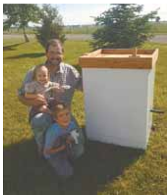
Philemon Riehl converted a used top loading washing machine into this cider maker. Bottom of washing machine drum is studded with nails that chop up apples.
