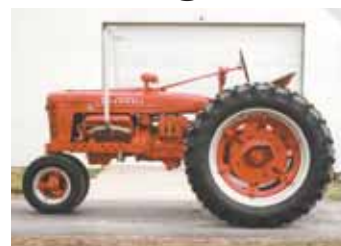
Larue Latimer repowered his 1940 Farmall H with the 304 cu. in., V-8 engine out of a 1975 IH 1-ton pickup.
