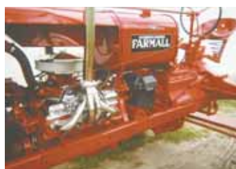
He installed chrome pipes on both sides of the tractor, fastening them to manifold headers turned upside down.
