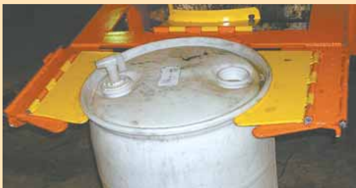
Barrel Grabber uses heavy-duty hinged metal wings to lock onto barrels by use of gravity. Wings automatically lock in place under barrel ring as operator raises unit. Another
