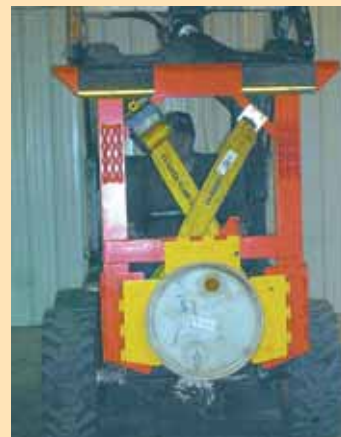
Winch and tie-down strap, bolted into one corner of Barrel Grabber’s frame, are used to pour. Strap wraps around barrel in a figure 8 design to keep it secure.
