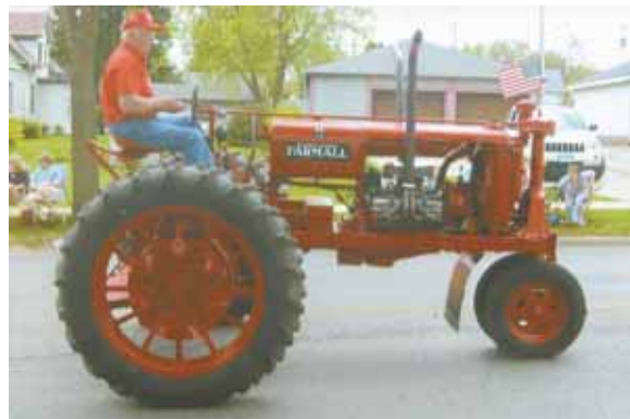
Glenn Buxengard installed a Chevy 350 cu. in., V-8 engine in his 1937 Farmall F-30 tractor. “There were a lot of challenges in making the conversion,” he says.
