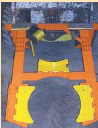
Winch and tie-down strap, bolted into one corner of Barrel Grabber’s frame, are used to pour. Strap wraps around barrel in a figure 8 design to keep it secure.
