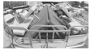
Pontoon folds up to an 8-ft. road width. Folded-out pontoon seats up to 17 people comfortably with room to spare.
