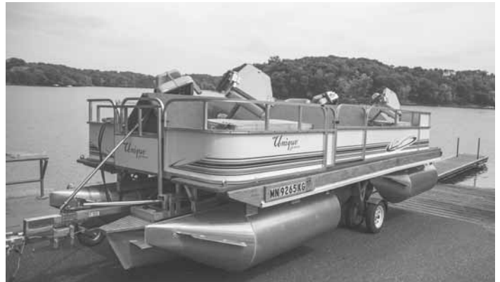
Fold-out pontoon extends from an 8-ft. road width to 11 ft. wide in the water. It has built-in wheels so no trailer is needed.
