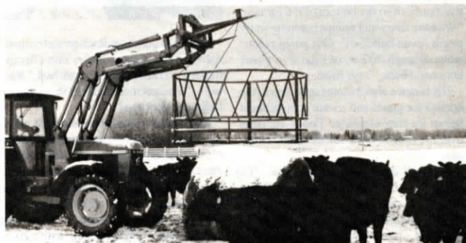
Four steel rods form the long "fingers" of the mover which attaches to the top of bale feeder.
