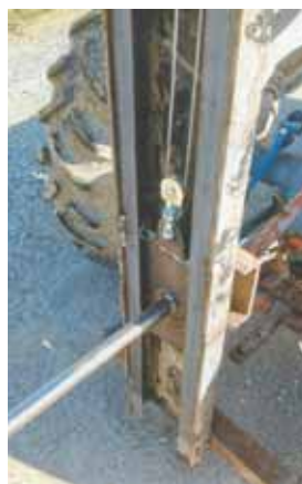
Huffman’s 3-pt. mounted “hay lifter” is designed to load and unload round bales. A small electric winch is used to raise and lower a steel plate with a bale spear welded to it. Plate rides inside a 7-ft. high post with a pulley on top of it.
