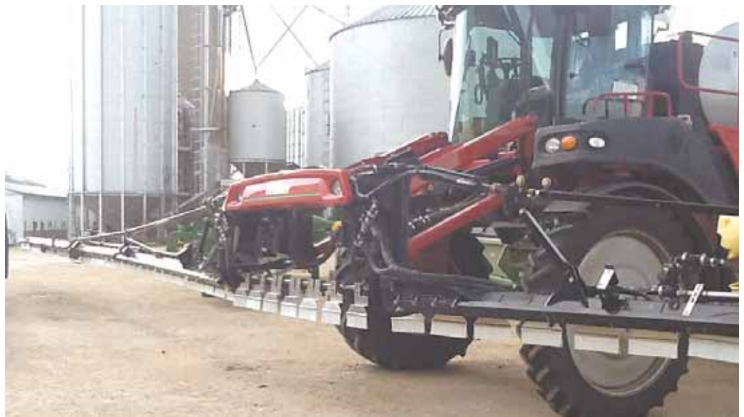
Pattern Master brushes are 6 1/2 in. wide with a thin layer of bristles that hang in front of boom’s spray tips. Wind striking the bristles is deflected, allowing the drops to form and fall intact.
