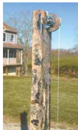
Huffman’s 3-pt. mounted “hay lifter” is designed to load and unload round bales. A small electric winch is used to raise and lower a steel plate with a bale spear welded to it. Plate rides inside a 7-ft. high post with a pulley on top of it.
