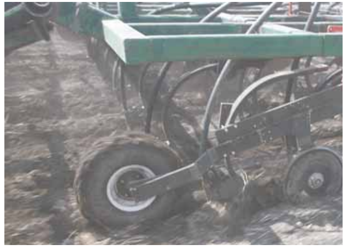
To install, the old shank is cut off and the existing opener is reattached to the side of the Orange Shank assembly. Optional coulters (shown above) can be mounted on the Orange Shank assembly bar ahead of the opener.
