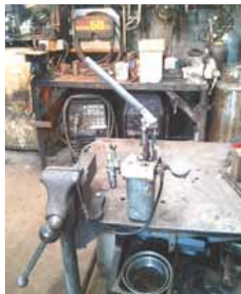
Fuel injector tester was made out of the hydraulic jack from a cab-over truck.
