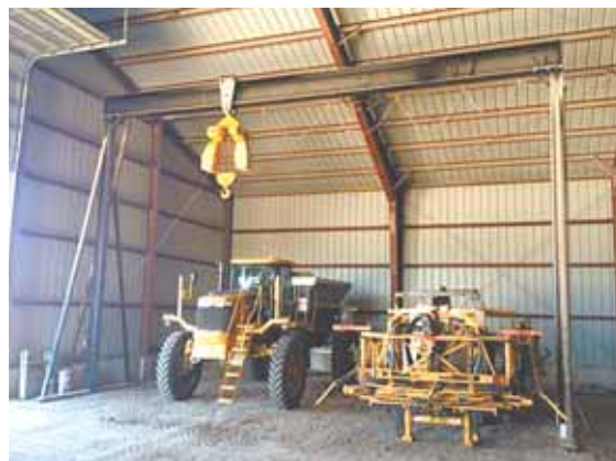
Andy and Tony Mulvihill's home-built crane stands 24 ft. tall, is 42 ft. wide and can lift 15 tons.
