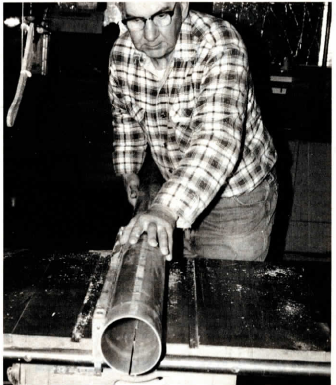
Tupper first cut the 4-in. dia. plastic pipe lengthwise into four equal-width strips.
