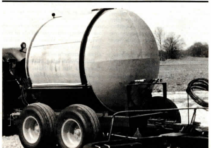
The 1,000 gal. sprayer can be ganged with any trailing implement without affecting the tractor's turning radius.
