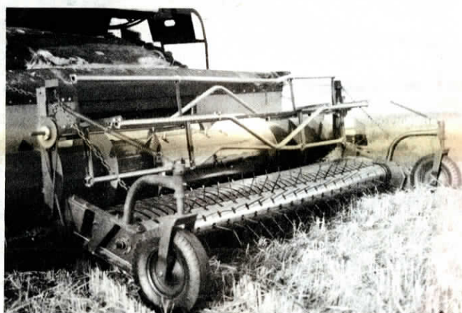
Reel forces crop directly into combine auger.
