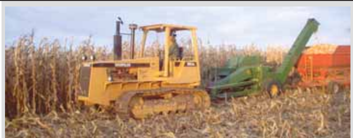
Repowered Deere/Cat crawler is shown here operating a 3-row corn picker in wet fields.
