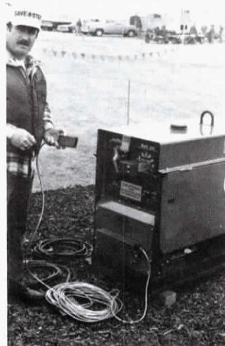
New control mounts outside the welder, requiring only 3 contact wires.
