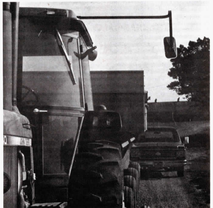
New extension mirror mounts vertically or horizontally, and slides in or out as needed.
