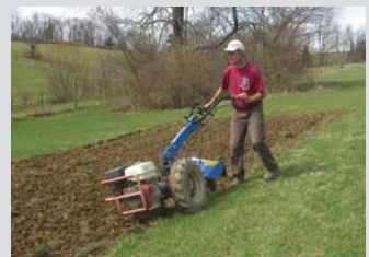
BCS tractor fitted with mower (above) and breaking sod with rotary plow (below).
