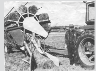
Eugene Tollakson's unusual bale wagon uses a big revolving reel to load small square or round bales.
