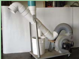
Blower Unit Cleans Cracked Nuts (Page 9)
