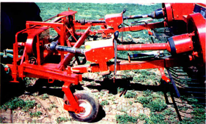
Baler behind tractor is driven by pto shaft mounted on hitch directly in line with tractor pto. Other baler is belt-driven by 9-ft. belt that rides on pair of 14-in. pulleys.
