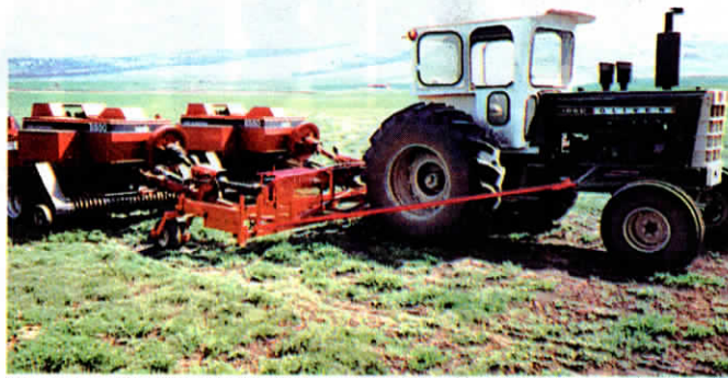
Pto-powered "splitter hitch" lets Story operate two Case-IH 8550 center feed balers at the same time.
