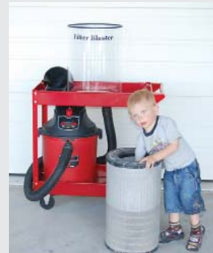
Air filter cleaner lets you use an air compressor to blow dust out of any canister-type filter.
