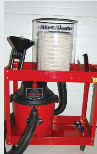
Unit comes with a cone-shaped, centrifugal force air induction chamber that pressurizes filter from the inside out.
