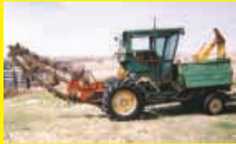
Home-Built Trencher Digs In Water Lines (Page 2)
