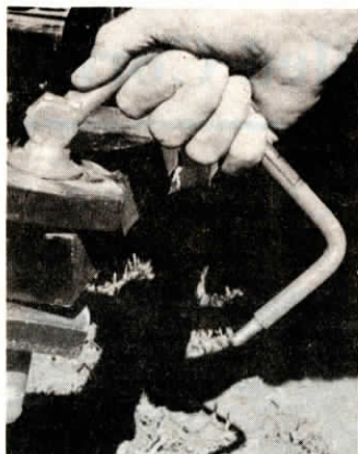
Pivoting handle hinges at the top and its bottom end inserts into a hole at the bottom of the pin. Cotter pin locks hinge so pin can't jump out.
