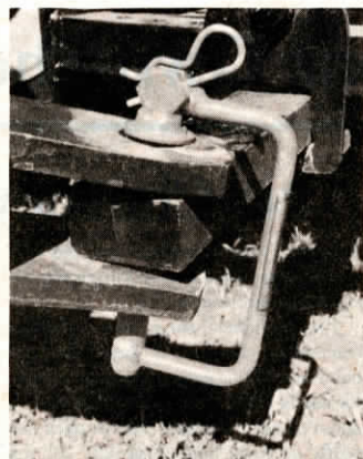
Pivoting handle hinges at the top and its bottom end inserts into a hole at the bottom of the pin. Cotter pin locks hinge so pin can't jump out.
