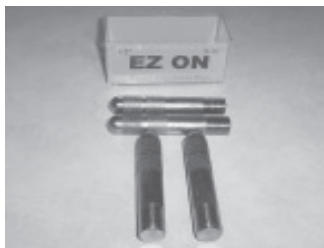
Kit includes two different sizes of alignment pins that make it easier to mount wheel on hub.
