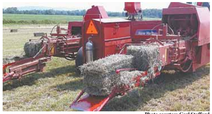
Double baler picks up hay from large merged windrows, separates the inflow into 2 separate chambers, and kicks bales out 2 separate chutes at the same time.
