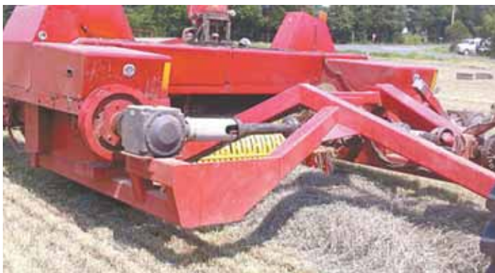
Rusty Inskeep cut up 2 New Holland 5070 balers and combined them into a single machine. “It lets us make more than 900 bales an hour in heavy, first crop hay,” he says.
