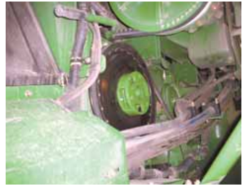
Special hub fits over the pulley of combine’s discharge beater, allowing you to use Lankota Inc. reversing tool to clean out a plugged beater.
