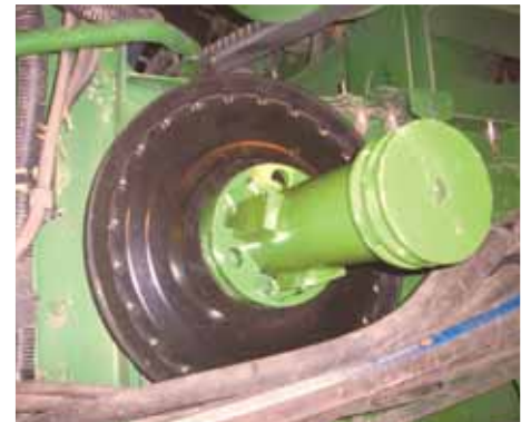
Photo shows reversing tool mounted on hub.
