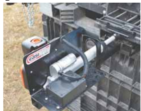
Remote-controlled seed box opener uses an electric actuator to open and close the slide gate on bulk boxes.
