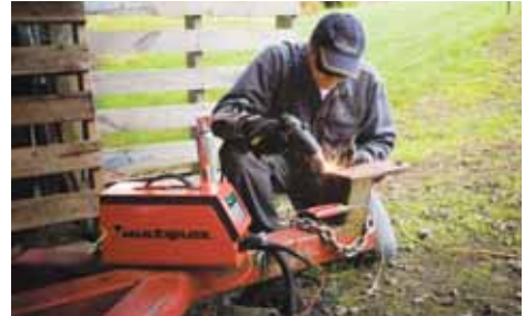
Not much bigger than an old-time radio, all the Multiplaz 3500 welder needs is 110 or 220-volt current, water and alcohol.
