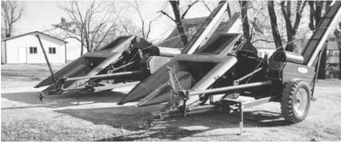
Reuben Zimmerman buys used New Idea corn pickers from farmers and rebuilds them, converting wide row models to narrow row.
