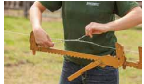
Deadends create a secure loop around a post or a radius around a corner post. Splices are said to be stronger than the original wire’s breaking strength.
