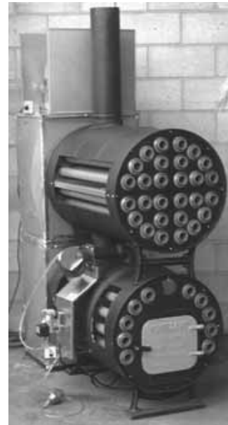
PapaBurn (with cutout sides to show heat exchanger tubes)
