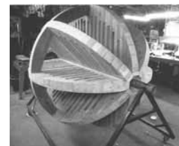
Taylor built the ball on a metal pipe that’s mounted horizontally, allowing him to spin the ball around as he built it.
