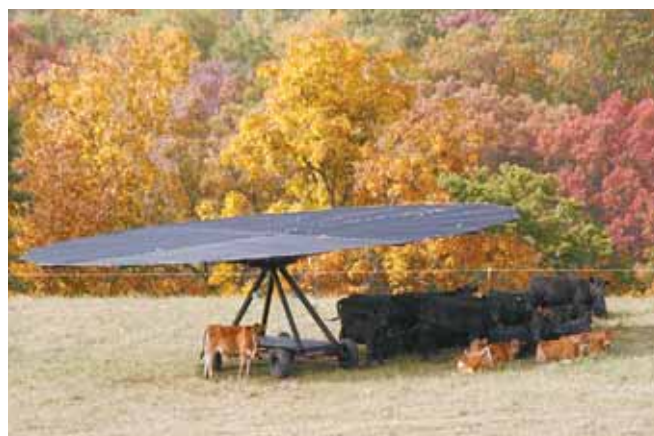
Portable 40-ft. dia. canopy is made of black poly shade cloth. It sets up in minutes and is easy to move.
