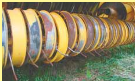
Baler pickup with bent, rusted steel bands.
