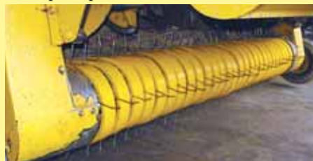
Pickup fitted with new Tobin poly bands.
