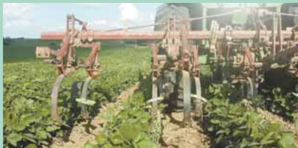
Photo at left shows a 4-row, 36-in. cultivator with the Flow-Shields angled away from the row, reducing the amount of dirt flowing into the soybean rows. Washers are used to center and firmly mount the Flow-Shields to “S” tine cultivator shanks (right).
