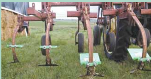
Photo at left shows a 4-row, 36-in. cultivator with the Flow-Shields angled away from the row, reducing the amount of dirt flowing into the soybean rows. Washers are used to center and firmly mount the Flow-Shields to “S” tine cultivator shanks (right).
