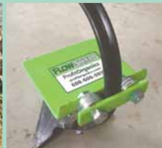
Photo at left shows a 4-row, 36-in. cultivator with the Flow-Shields angled away from the row, reducing the amount of dirt flowing into the soybean rows. Washers are used to center and firmly mount the Flow-Shields to “S” tine cultivator shanks (right).
