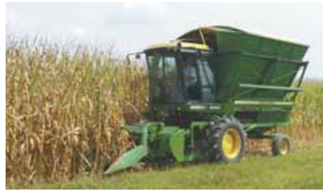
"It was a challenge, but an enjoyable one," says Jim Anderson, who converted a used Deere 9920 cotton picker into a silage chopper equipped with a dump box.
