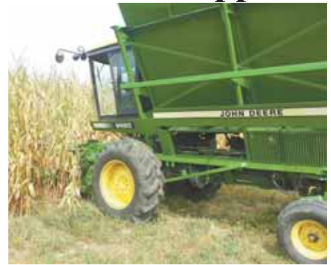
To improve visibility, he lowered the cab by about 6 in. The cotton basket was replaced by a side-dump box from a silage wagon.
