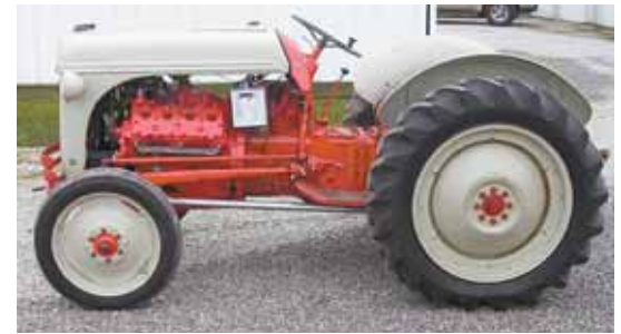
Kit costs $1095 and contains all the hardware needed to connect the V-8 engine and clutch assembly to the Ford 8N transmission and frame. Knasel says it takes about 8 to 10 hours to install.
