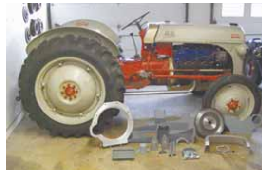
Photo shows parts included in overhead valve conversion kit for N-Series Fords.
