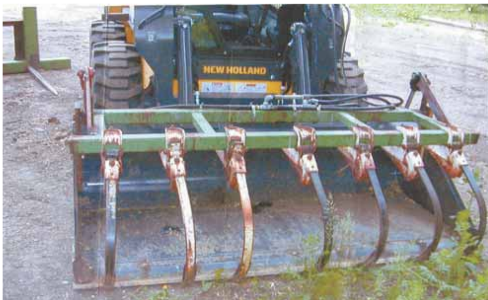
Harlen Grovom used part of the frame and some shanks from an old field cultivator to build this grapple fork. He bolted it to the bucket on his New Holland skid loader.
