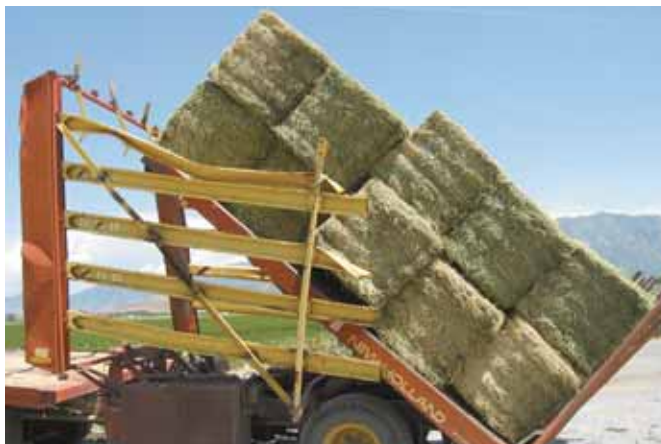
Garry Brown modified his self-propelled small bale stacker wagon to haul and stack up to 10 big square bales at a time.
