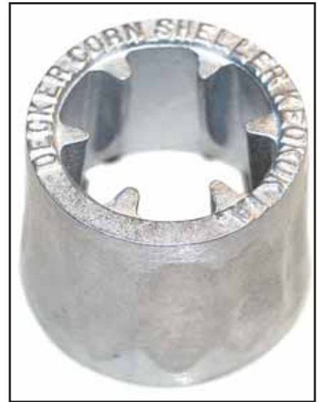
To use the mini sheller, you twist the ear through the collar and let sheller’s 6 ridges rub the kernels off.
