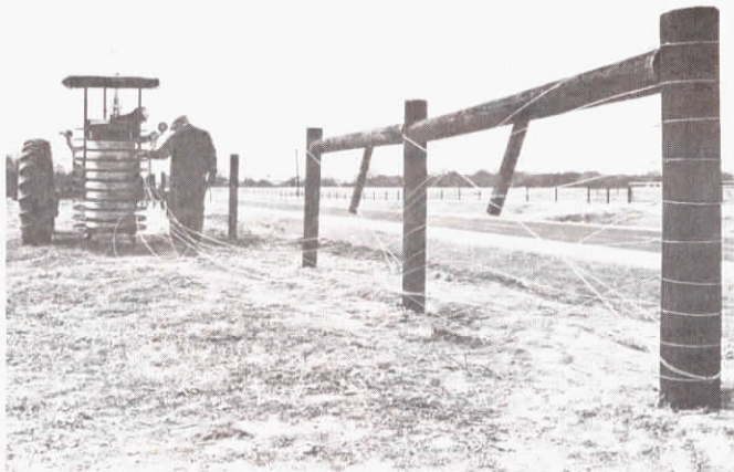
New multi-reel fencer can unroll up to 10 high-tensile wires at one time. Its inventors hail from New Zealand.
