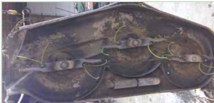
Pairs of 18-in. long weed trimmer lines loop through holes that Steven Simpson drilled into the mulching blades on his Deere riding mower.
