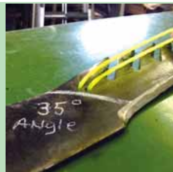
Simpson drilled the line mounting holes at about a 35 degree angle to the blade, which keeps the lines spaced about 1/4 in. apart.
