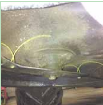
Simpson drilled the line mounting holes at about a 35 degree angle to the blade, which keeps the lines spaced about 1/4 in. apart.
